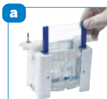
Insert glass plates between pressure frame and gasket
