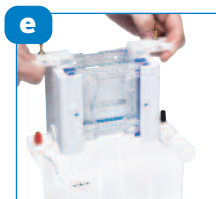
Transfer to tank and fill with buffer
