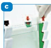
Insert a gel cassette into each side of the inner buffer chamber in the PAGE insert, and begin tightening the vertical screw-pins.
