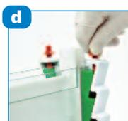
Continue to tighten the screw-pins until the gel clamps glide out of the resting slots and fix firmly against the glass plates pushing them upright.
