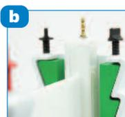
Loosen the vertical screwpins in the PAGE insert to release the locking mechanism, allowing the gel clamps to sit in the resting slots.
