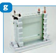
Pour in the gel solution, insert the combs and allow the wells to polymerise.
