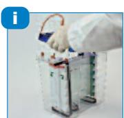
Replace the lid, connect the power supply and run.
