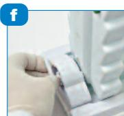
Insert cams and turn until tight, drawing the PAGE insert onto the casting to form a leak-proof seal.
