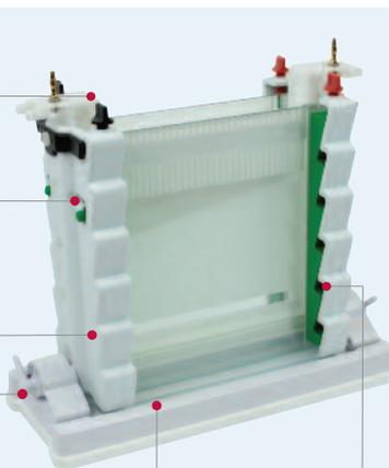
Flat, level gasket prevents current leakage from inner buffer chamber
