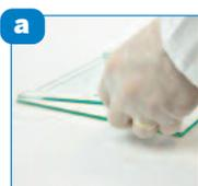
Assemble each gel cassette on a flat level surface, by placing the plain glass plate down with the spacers facing upwards followed by the notched glass plate.
