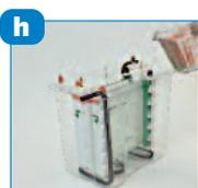
Transfer the PAGE insert to gel the tank. Fill the inner and outer buffer chambers before loading samples.
